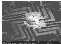
Fig. 2. Lamella placed on prefabricated substrate.
